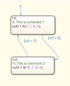
When you generate Verilog code from the model, HDL Coder displays the comments in the Stateflow Chart inline beside the corresponding Stateflow object.
