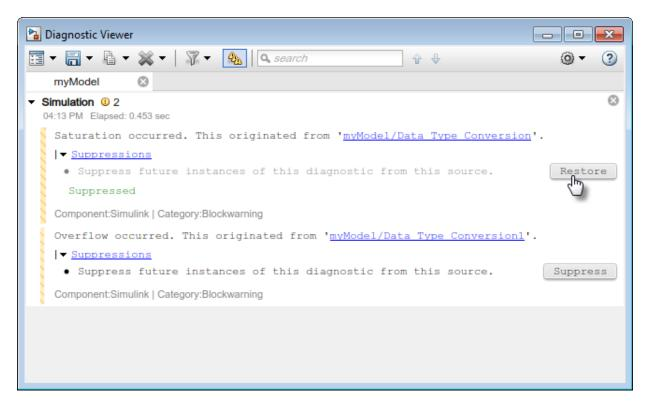
You can also control the suppressions from the command line. To view the existing suppressions on the model, use the Simulink.getSuppressedDiagnostics function.
